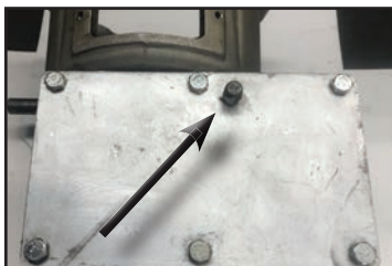
Fig. II Vent location with correct cover orientation
