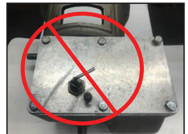
Fig. V The vent will leak from this ruined cover.
