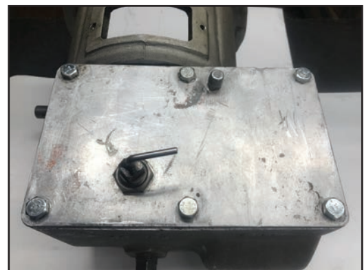
Fig. V The vent will leak from this ruined cover.
